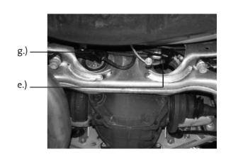
■ Disconnect shock absorber from track control arm ②.
