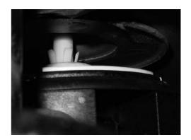
■ Mount equalizing reservoir (torque to 20 Nm) ③.
